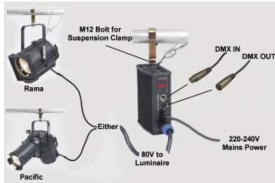
80V DMX power supply connection diagram
