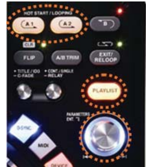
Loop (also as Hot Start), Play List, (switch File Play & Play List mode), Parameter Knob (Music Search, Pitch Control Pre-Setting, etc.)
