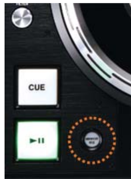
Mirror Mix – adjust tempo and signal coming out from Deck A & B (like Double disc play)
