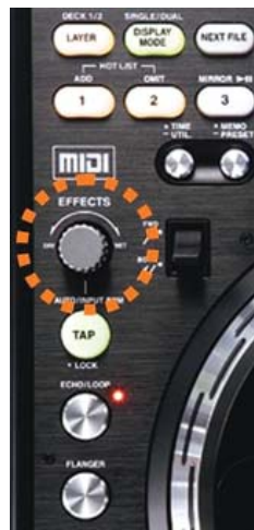
Effects Knob – Echo/Loop, Flanger, Filter (Filter Effects has High/Mid/Low Pass by adjusting Wet-Dry Knob)
